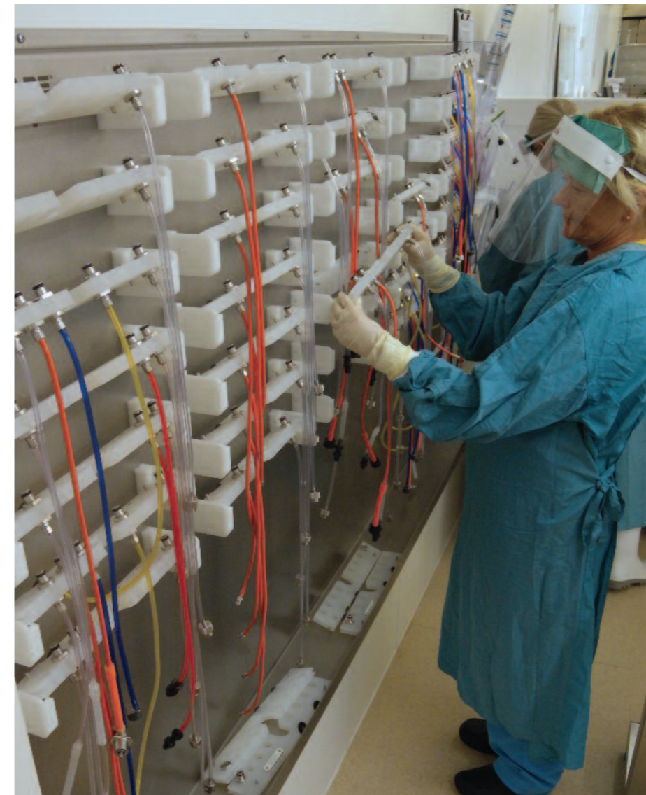
Neocare's 'hook-up organiser' is a purpose-made rack housing the AER's manifolds and tube assemblies for the various types of scopes
